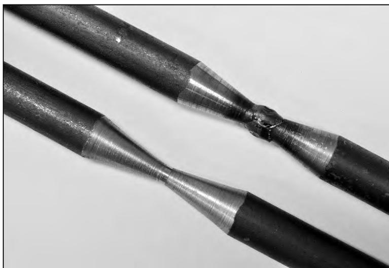
Fig. 2. Test specimens #3 and #4 - rotationally symmetric double U butt welded joint and massive element without welding
