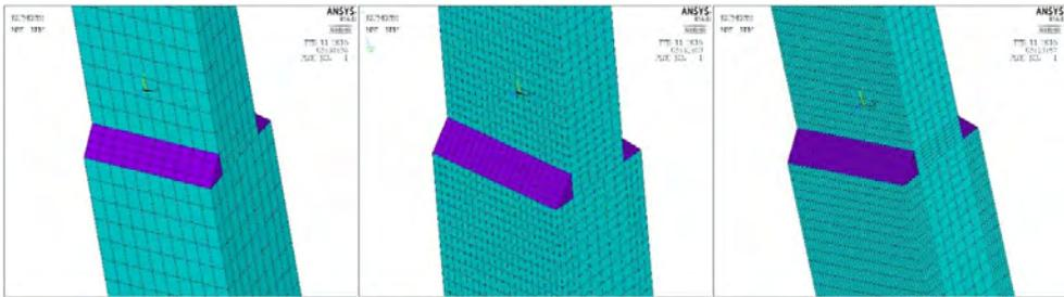
Fig. 3. Numerical model with various FEM mesh density of test specimen #1 - fillet welded lap joint
