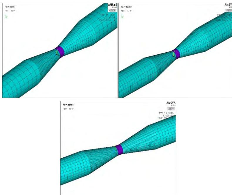
Fig. 5. Numerical model with various FEM mesh density of test specimen #3
