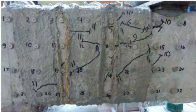
Fig. 8. Distribution of cracks on the surface of the strengthening
