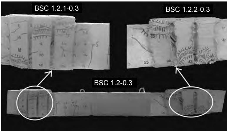
Fig. 5. The tested strengthened beam BSC 1.2-0.3
