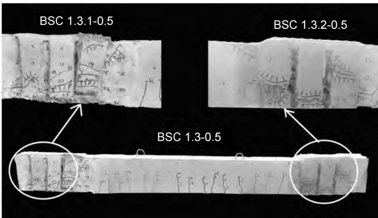
Fig. 6. The tested strengthened beam BSC 1.3-0.5
