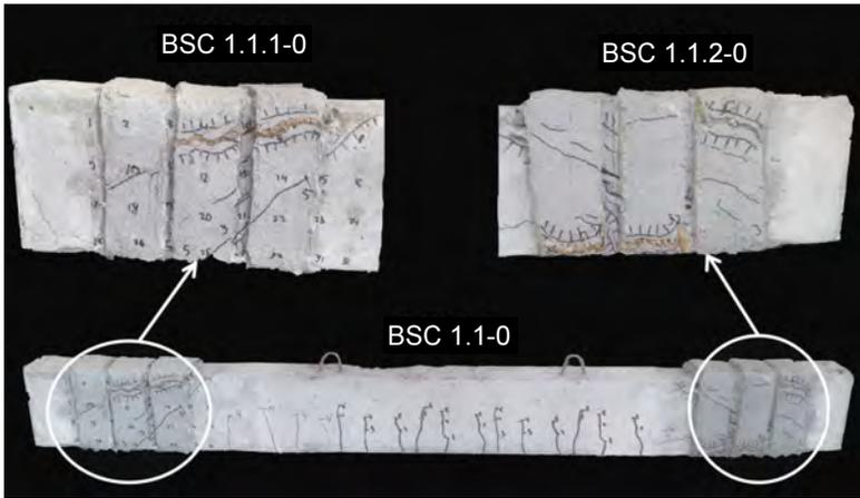
Fig. 4. The tested strengthened beam BSC 1.1-0
