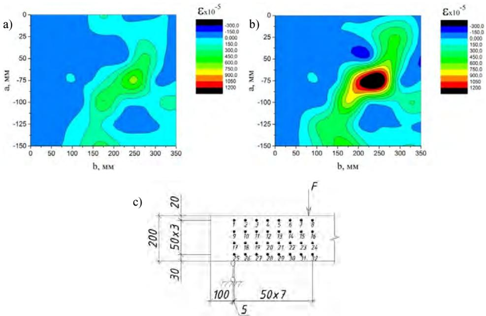
Fig. 3. The distribution of concrete deformation in the shear area for beam BO-1.1:
