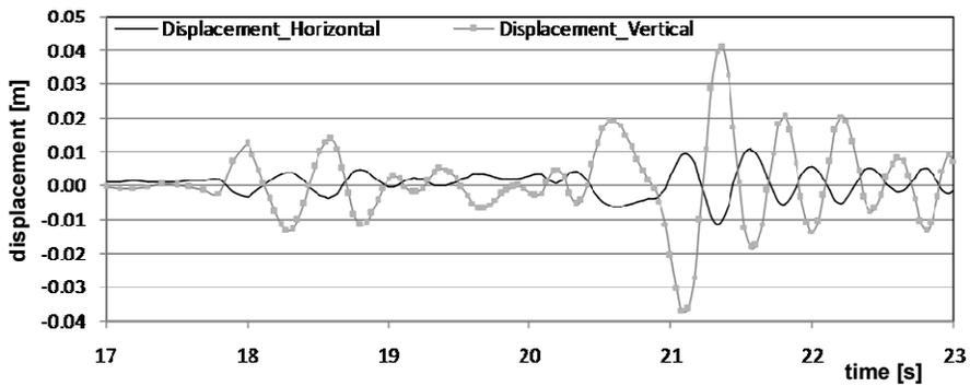
Fig. 6. Time dependent response of the horizontal and vertical displacement of fluid in "RTEF" point
