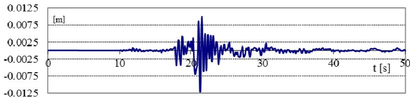
Fig. 4. Input time dependent horizontal displacement measured during of earthquake Loma Prieta
