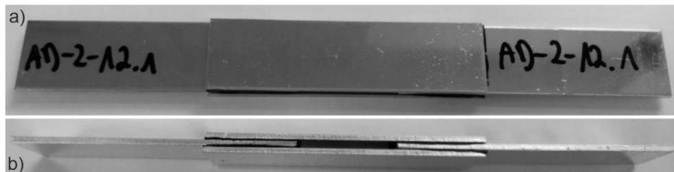
Fig. 4. Photos of exemplary joint: a) top view, b) side view
