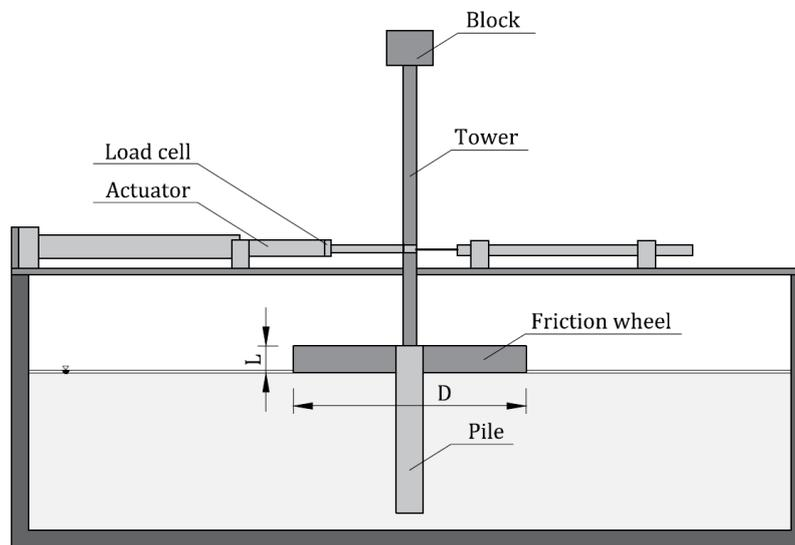
Fig. 6. Cross-sectional view of the analyzed hybrid pile model. The drawing was made on the basis of the article [12]
