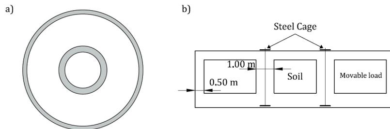
Fig. 1. Foundation footing with active stabilization system; a) plan view, and b) cross section. [5]
