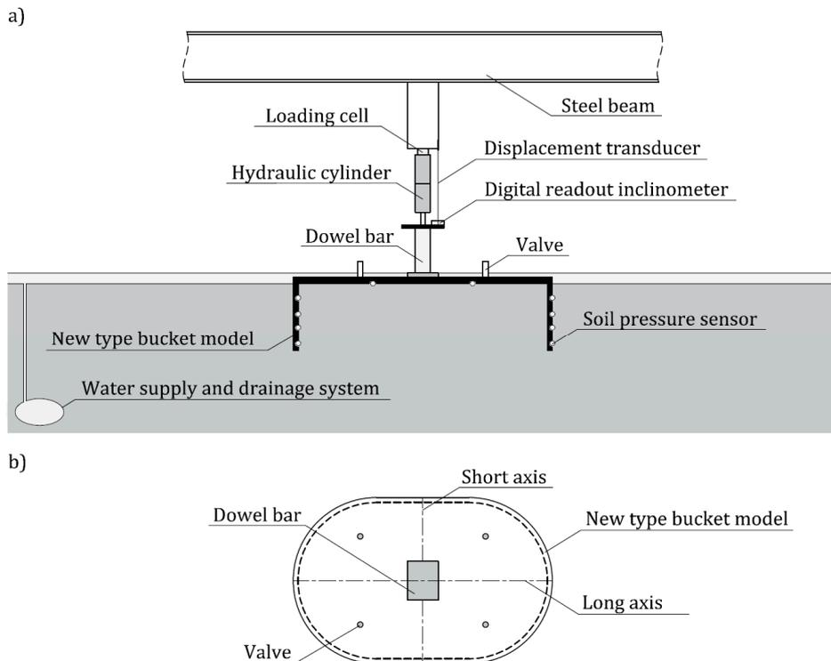
Fig. 3. Scheme of a new bucket foundation type; a) elevation view of test package; b) view from above. The drawing was made on the basis of the article [4]
