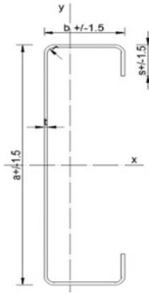
**Fig. 1.** Cross-section of a C-profile C140:  $a = 140$  mm,  $b = 38$  mm,  $s = 18$  mm,  $t = 1,5$  mm,  $r = 3$  mm
