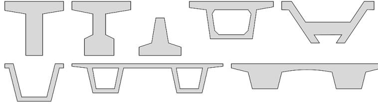
Fig. 1. Examples of shapes of compressed elements [1]
