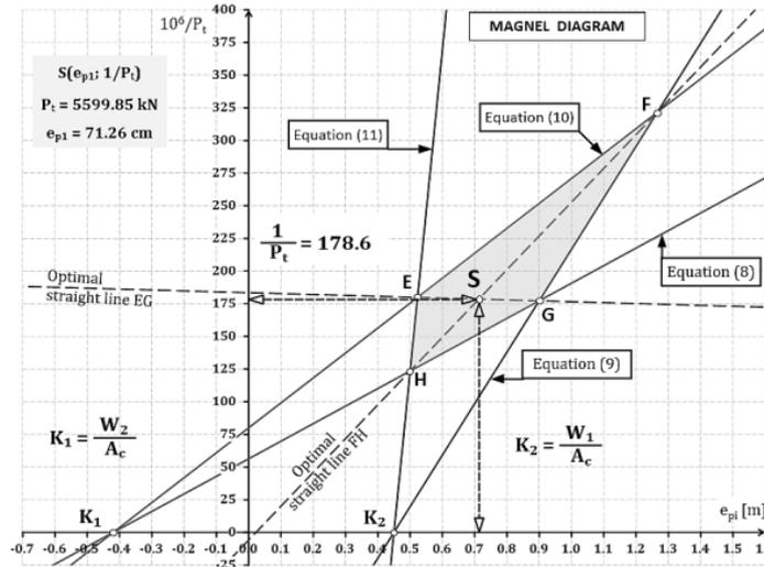
Fig. 3. The final graphic solution of the modified Magnel method
