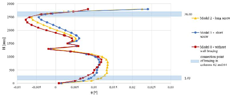
Fig. 9. The course of variability of the torsion angle along the length of the column web 64
