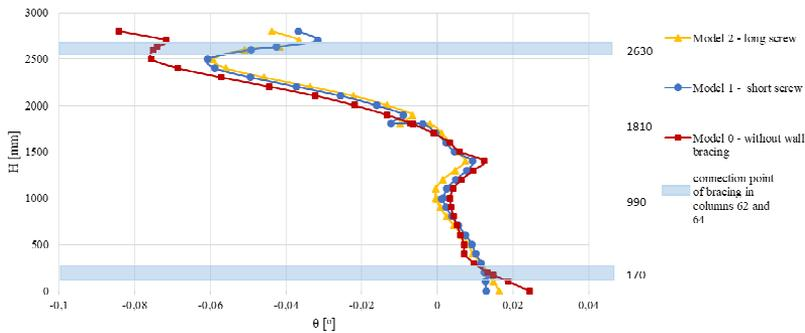
Fig. 8. The course of variability of the torsion angle along the length of the column shelf 63
