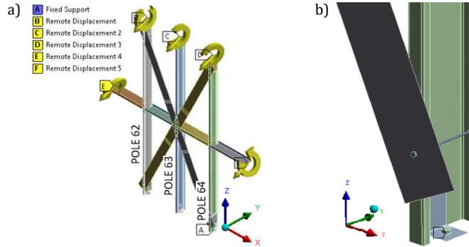
Fig. 4. Boundary conditions of the analyzed section: a) displacements applied at the center of gravity of the cross-section of the profiles, b) support in the form of anchoring the M10 anchor (example of a long bolt connection)
