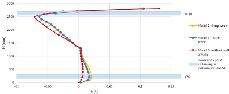
Fig. 5. The course of torsion angle variability along the column web length 62
