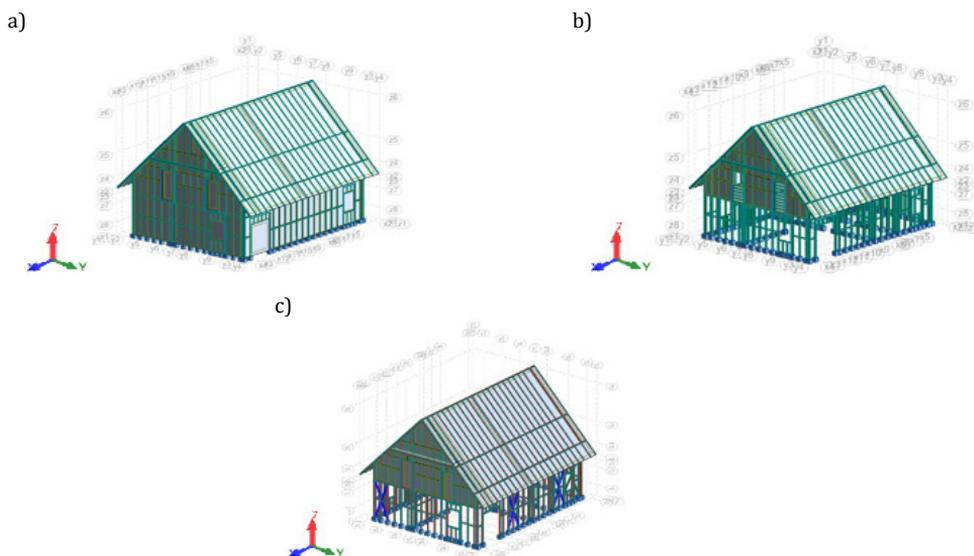
**Fig. 1.** Calculation models adopted: a) Model I - building structure with all sheathing, b) Model II - building structure without stiffening plated on the ground floor, c) Model III - building structure without stiffening plates on the ground floor, with vertical bracing
