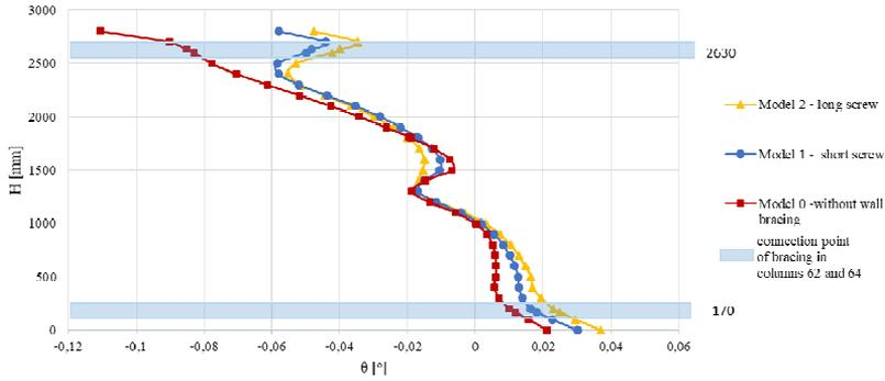
Fig. 6. The course of torsion angle variability along the length of the column shelf 62
