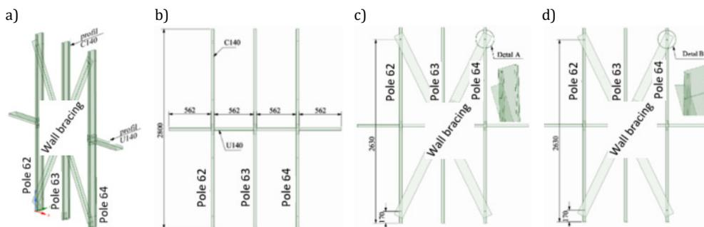
**Fig. 3.** Diagram of the wall section being analyzed: a) general view of selected profiles, b) Model 0 without bracing, c) Model 1 with bracing attached to one of the profile shelves (detail A), d) Model 2 with bracing attached by two profile shelves (detail B)
