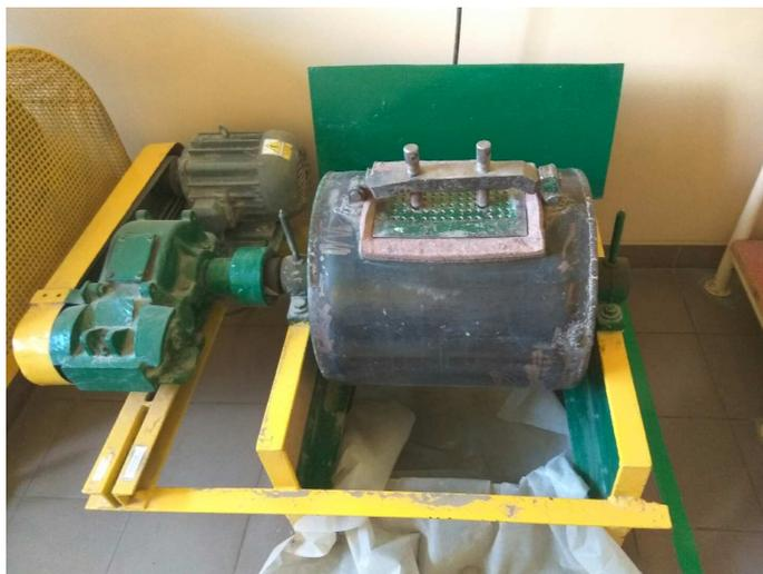
**Fig. 1.** Laboratory ball mill
