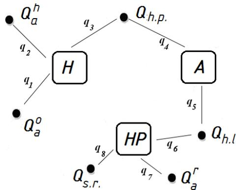
Fig. 2. Oriented graph of heat containers of solar air heater
