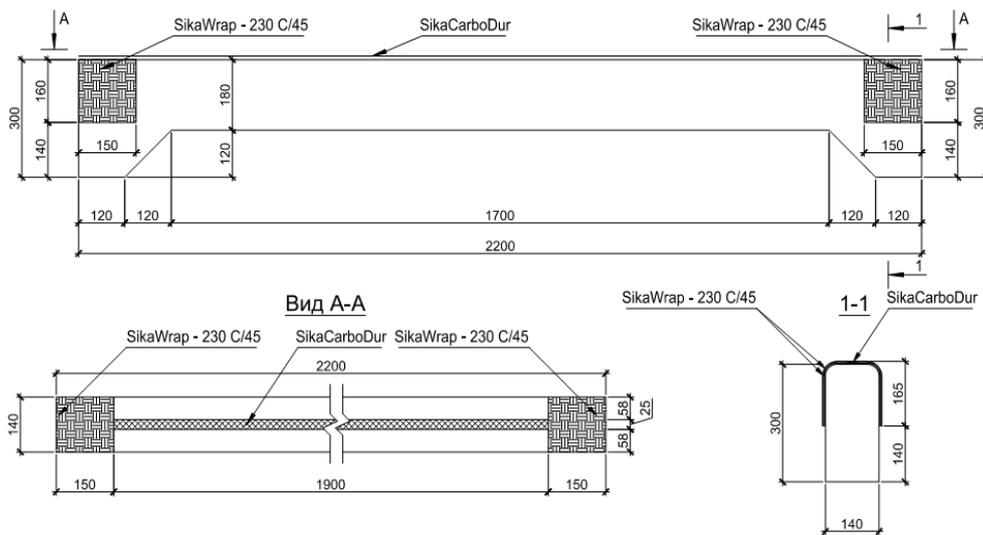
Fig. 3. Reinforcement of samples strengthened by carbon laminate
