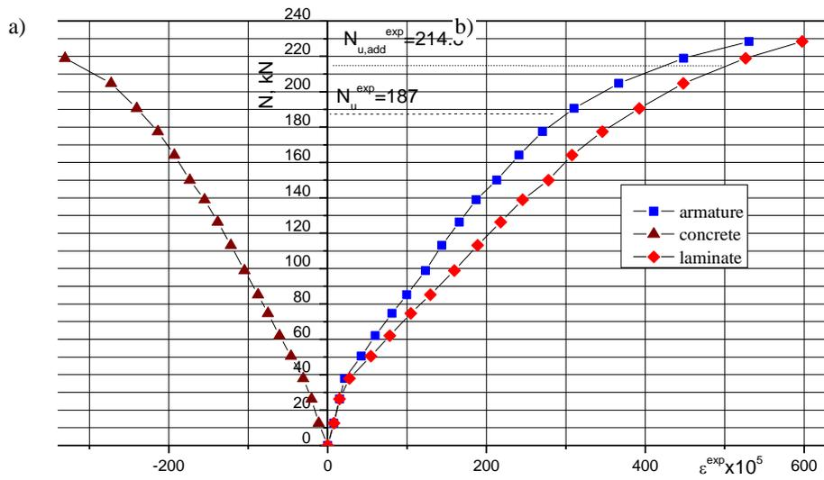
Fig. 11. Strain in stretched reinforcement (armature), laminate and compressed concrete of column CSL-2.11
