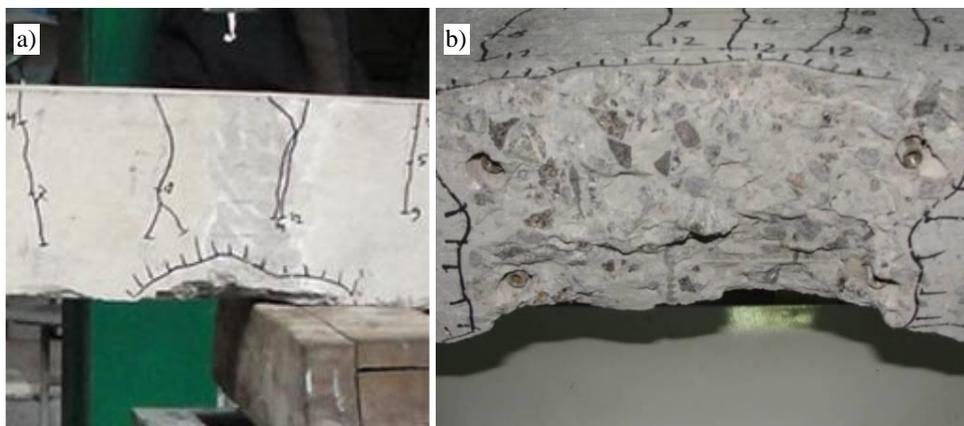
Fig. 7. Compressive area of columns CU-0.1 (a) and CU-0.2 (b) after failure
