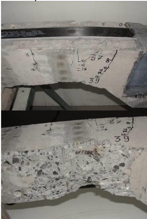
Fig. 12. Compressive area of column CSL-2.11 after failure. Side view (a), bottom view (b)
