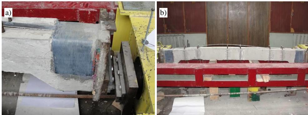
Fig. 9. The character slipping of the laminate from anchoring in a sample CSL-1.3. In place of anchoring (a), general view (b)
