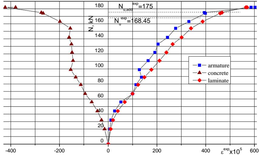
Fig. 8. Strain in stretched reinforcement (armature), laminate and compressed concrete of columns CSL-1.3 and CSL-1.4 (CSL-1 - average of twins)
