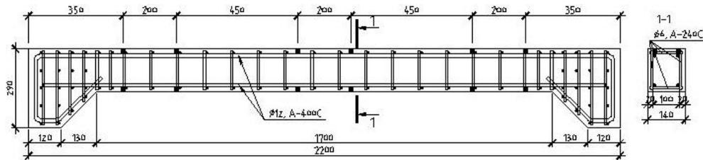
Fig. 1. Design and reinforcement of unstrengthened samples
