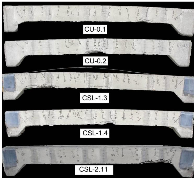
Fig. 13. Columns CU-0.1, CU-0.2, CSL-1.3, CSL-1.4, CSL-2.11 after testing
