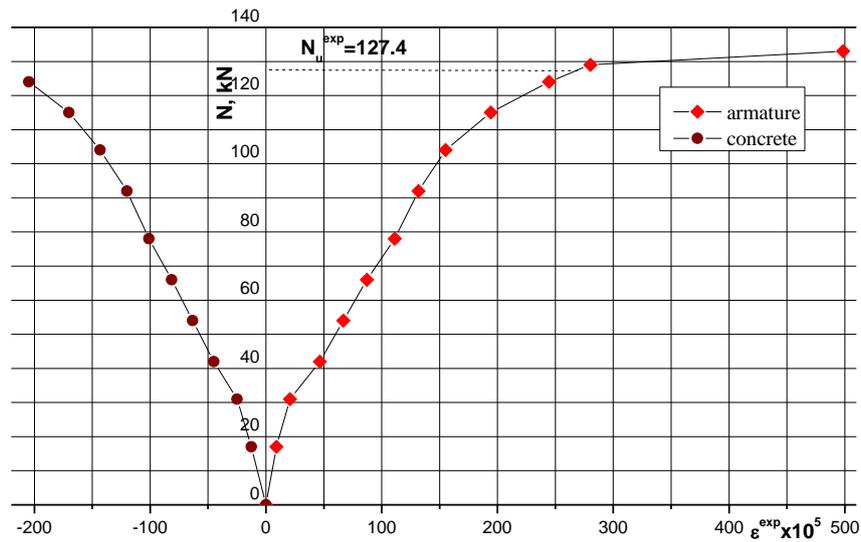
Fig. 6. Strain in stretched reinforcement (armature), compressed concrete of unstrengthened columns CU-0.1 and CU-0.2 (CU-0 - average of twins)
