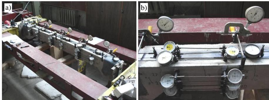
Fig. 5. Strengthened sample during test. The general view (a) and first cross-sections (b)
