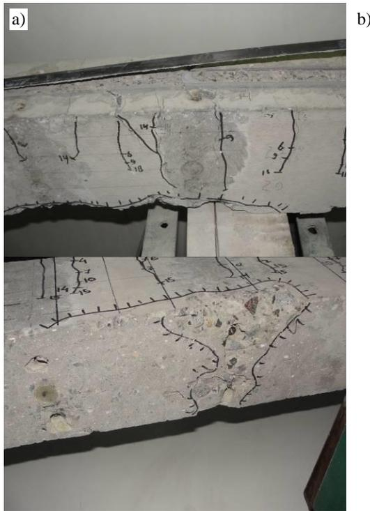
Fig. 10. Compressive area of columns CSL-1.3 (a) and CSL-1.4 (b) after failure
