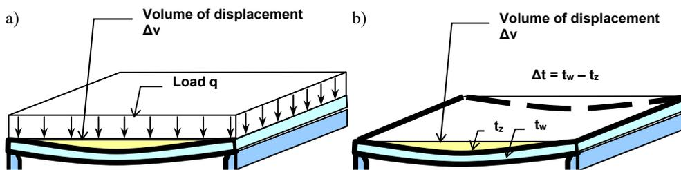
Fig. 3. Volume of a single glass sheet displacement with: a) surface load, b) temperature load
