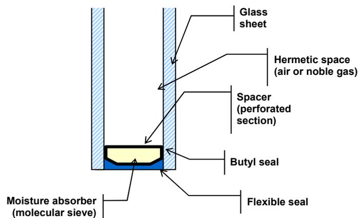
Fig. 1. Diagram of the complex glass panel construction with two-stage sealing
