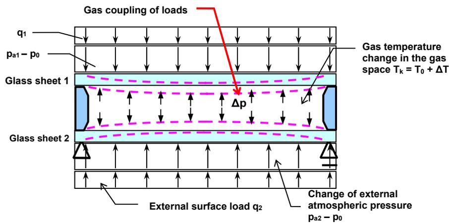
Fig. 4. Diagram of glass sheets load in a hermetic unit
