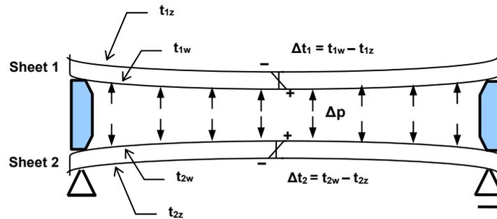
Fig. 7. Gas couplings of loads caused by temperature changes in both glass sheets
