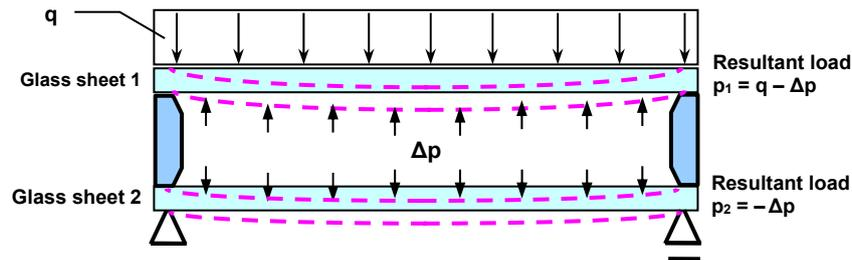
Fig. 5. Diagram of transmitting surface load between glass sheets of a glass unit
