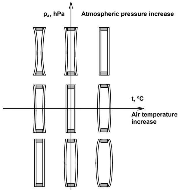
Fig. 2. Displacement of glass sheets in a glass unit caused by climatic factors [4]
