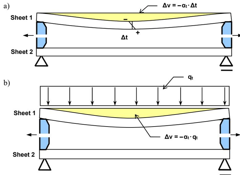
Fig. 6. Volume of displacement caused by linear (in glass thickness) temperature changes with a gas space without a hermetic seal: a) actual load, b) substitute surface load
