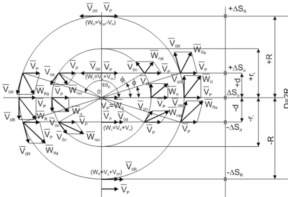
Fig. 2. Variation of the resultant velocity depending on  $\omega_i = v_p + v_{0i}$  ( $r_i = 0, \dots, R$ )
