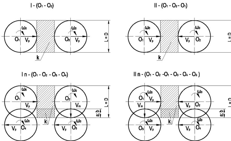
Fig. 3. Computation schemes for different variants of the disk axis path in surface treatment.
