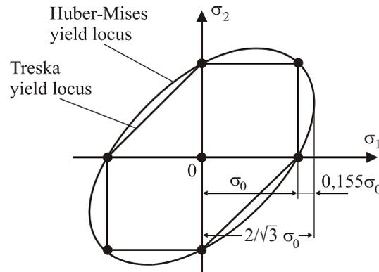
Fig. 9. Comparison of the Huber-Mises and the Treska yield criteria on a plane  $\{\sigma_1, \sigma_2\}$
