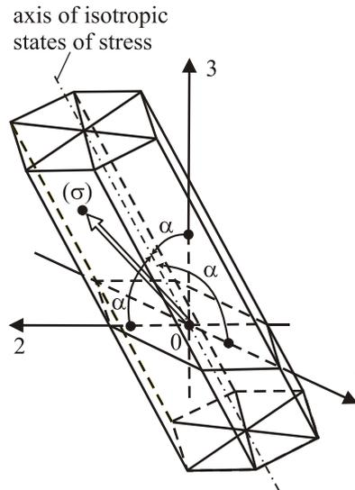
Fig. 6. The Treska yield criterion in the space  $\{\sigma_i\}$
