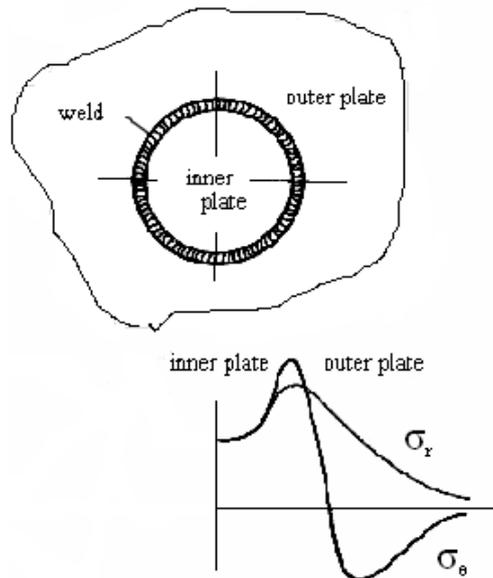
Fig. 3. Residual stresses in a circular patch weld
