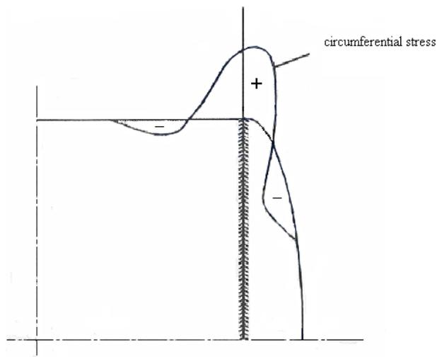
Fig. 5. Residual stresses in a cylindrical tank
