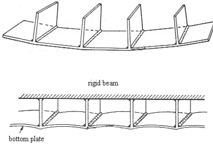
Fig. 3. Types of distortion in fillet-welded structure
