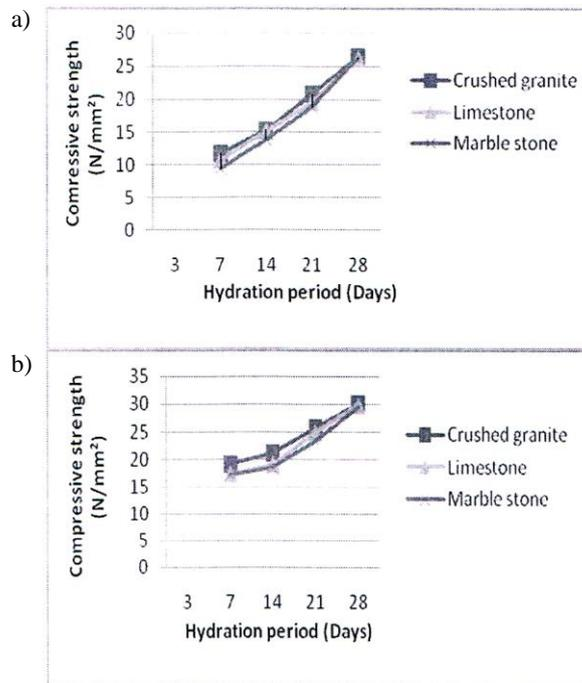
Fig. 1. Compressive strength of the concrete produced from the various coarse at water cement ratios of: a) 0.5 and b) 0.6, and design concrete strengths of 20 N/mm<sup>2</sup>
