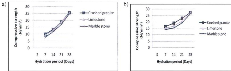
Fig. 2. Compressive strength of the concrete produced from the various coarse aggregate at water cement ratios of (a) 0.5 and (b) 0.06, and design concrete strengths of 30 N/mm<sup>2</sup>
