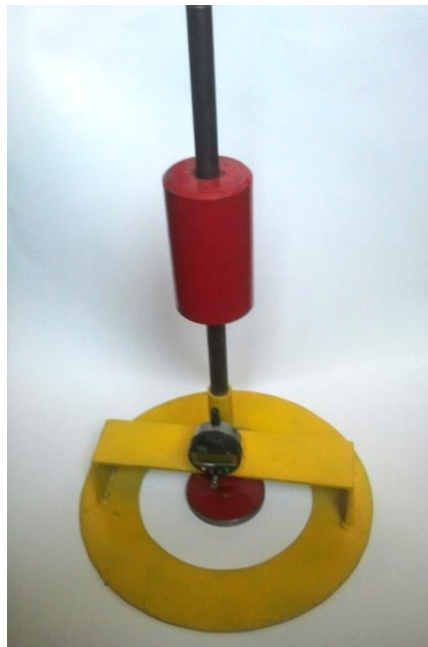
Fig. 1. Device for measuring of the changes in consistency properties on the surface of the formed concrete
