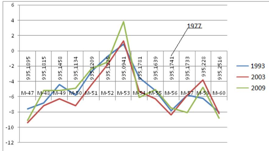
Fig. 3. Observation chart of settling marks outside the walls of special building
