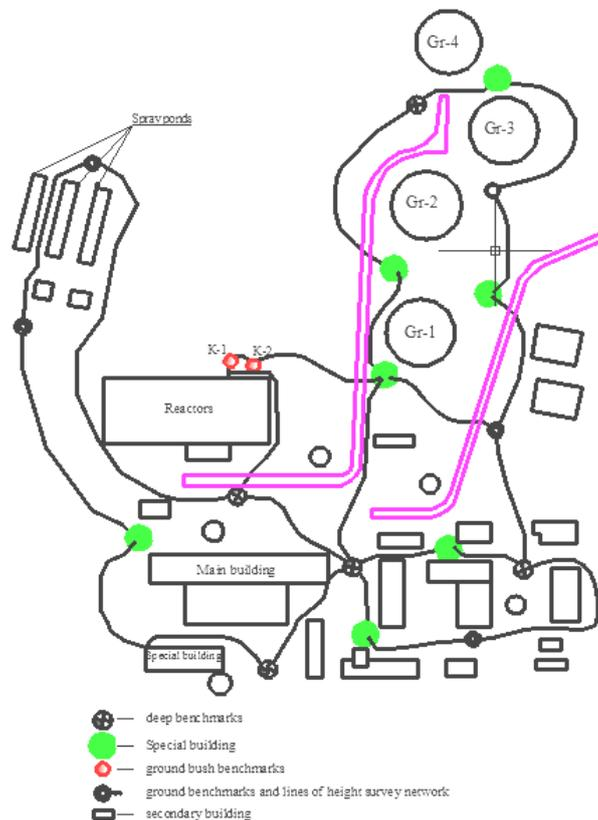
Fig. 2. The scheme of structures and height network of ANPP
