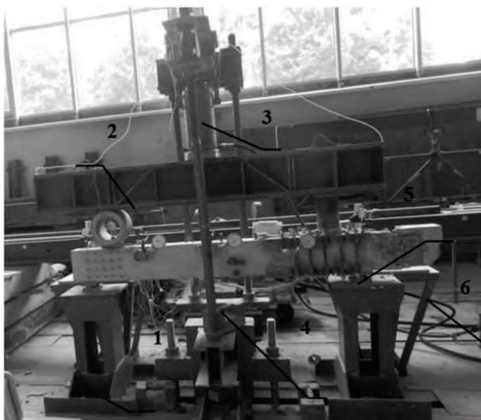
Fig. 6. Testing second inclined cross-section: 1 - support, 2 - distributive metal beam, 3 - hydraulic crank, 4 - testing beam, 5 - metal jacket, 6 - crashed cross-section
