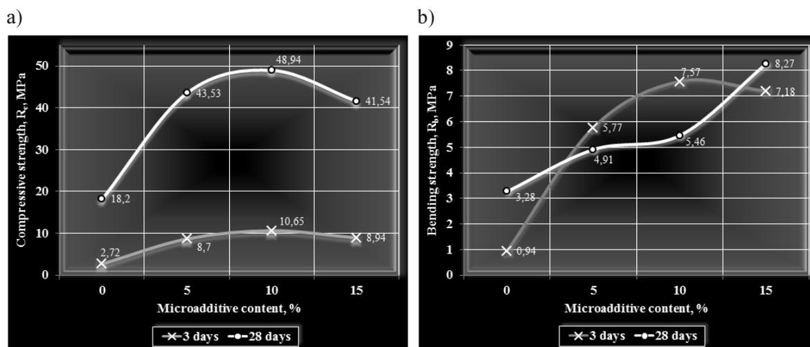
Fig. 2. Tensile strengths of the fine-grained concrete depending on the microadditive on the basis of silica sand content: a) under compression, b) under bending
