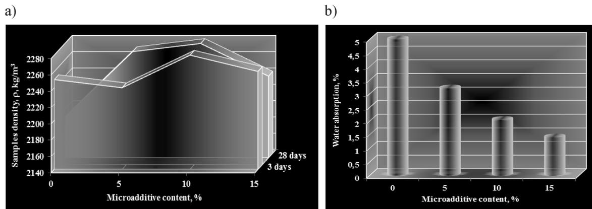
Fig. 3. Dependence of the fine-grained concrete samples from the content of the integrated organic-mineral additive: a) density, b) water absorption
