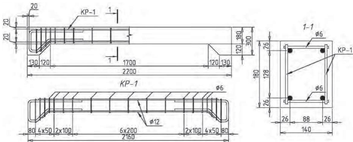
Fig. 1. Column dimensions and reinforcement drawings
