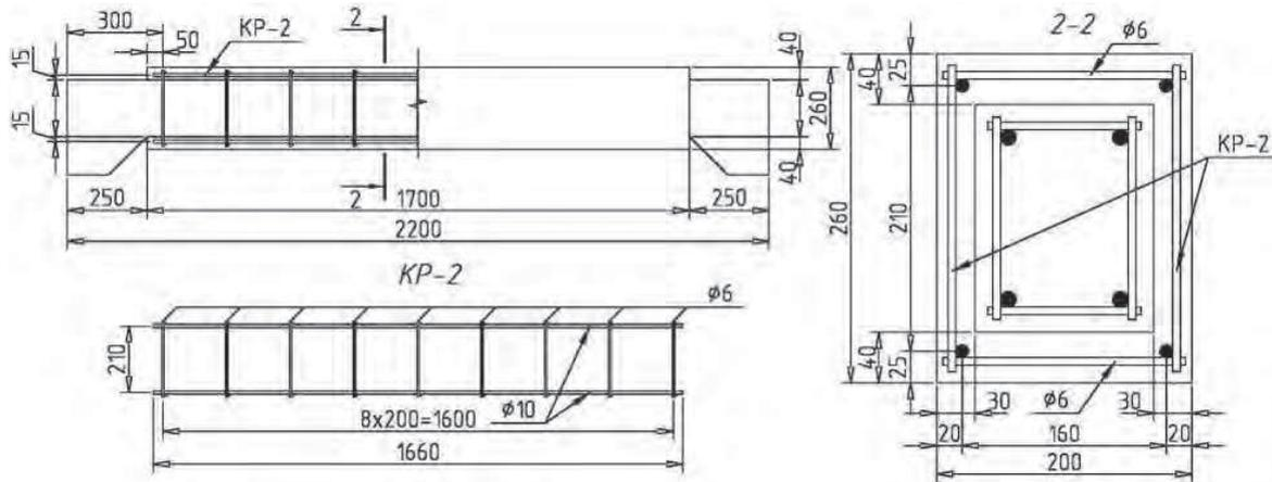
Fig. 2. Strengthened column dimensions and reinforcement drawings
