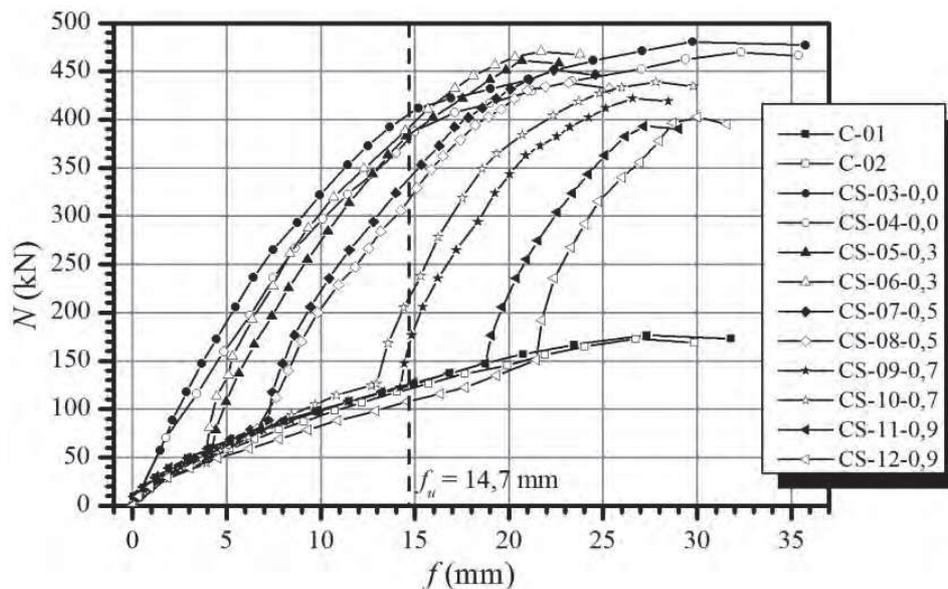
Fig. 3. Load vs midheight deflection graphs for tested columns
