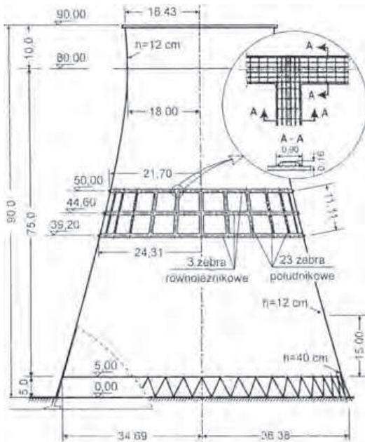
Fig. 7. The strengthening of the cooling tower shell by reinforced concrete ribs - the first variant [9]
