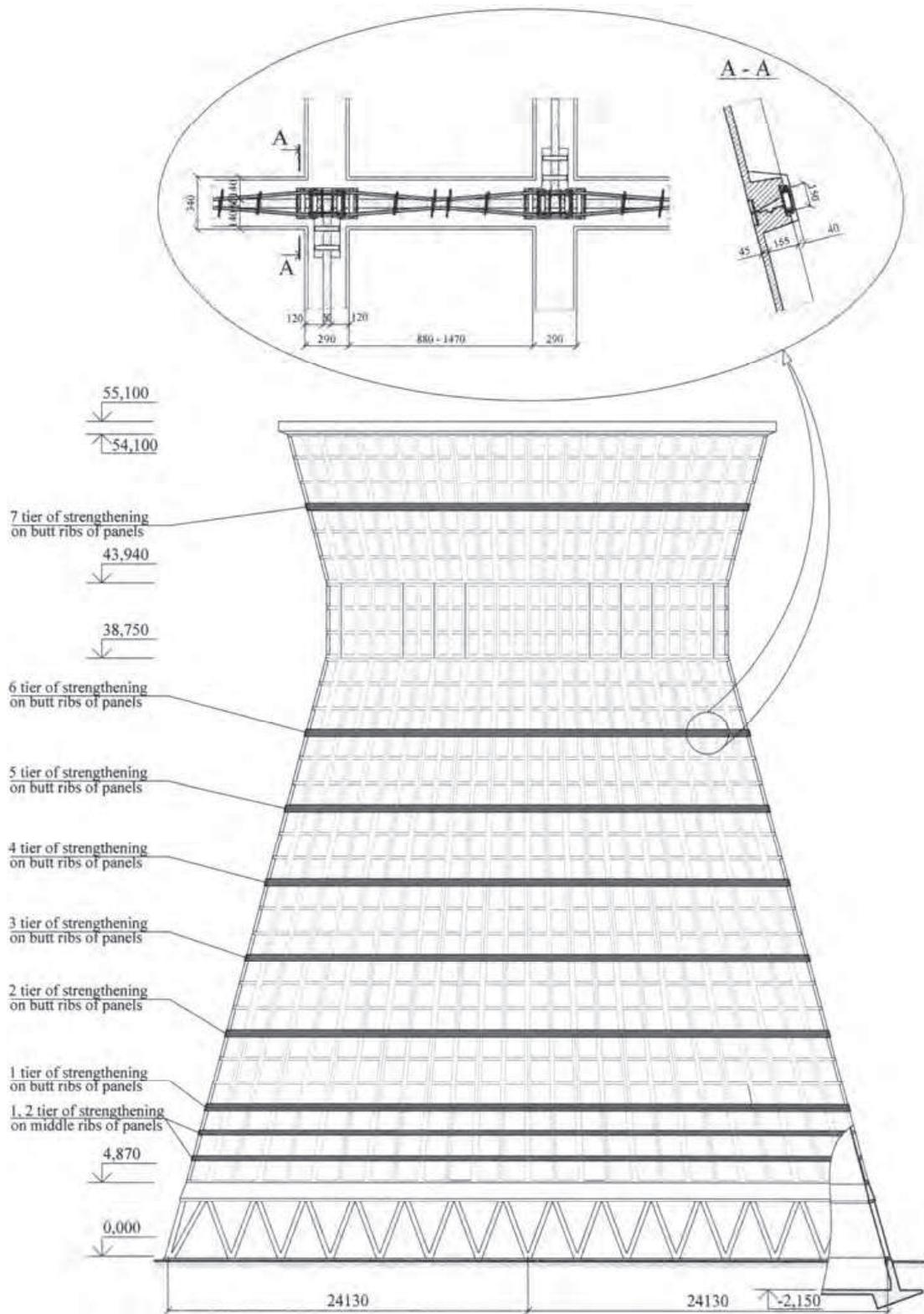
Fig. 3. The storeys of strengthening the horizontal ribs of precast reinforced concrete panels of cooling tower shell by prestressed ring armature
