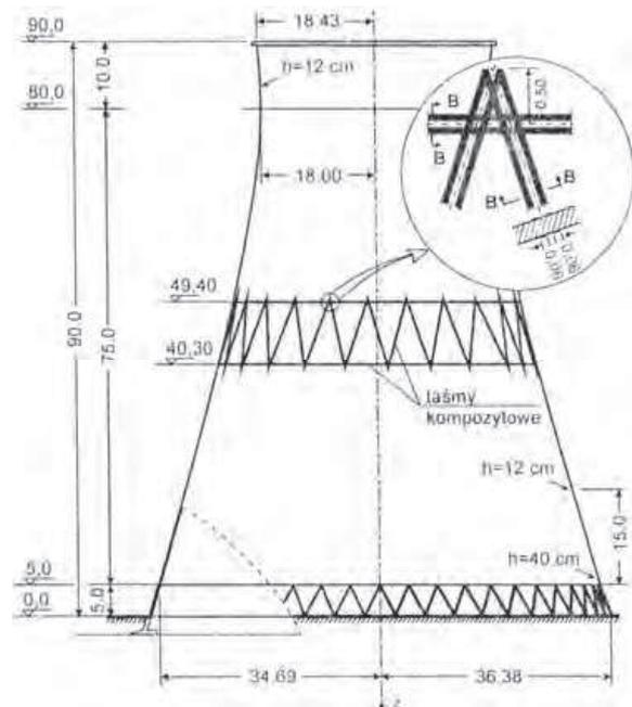
Fig. 8. The strengthening of cooling tower shell by composite tapes - the second variant [9]
