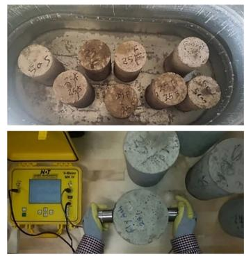
Fig. 1. Concrete samples and UPV test
