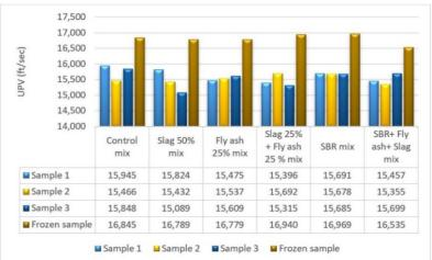
Fig. 4. Damage levels and average UPV values
